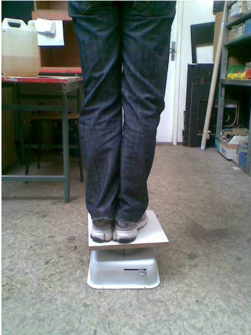
This aluminum stove withstood a 100 kg deformation test.
