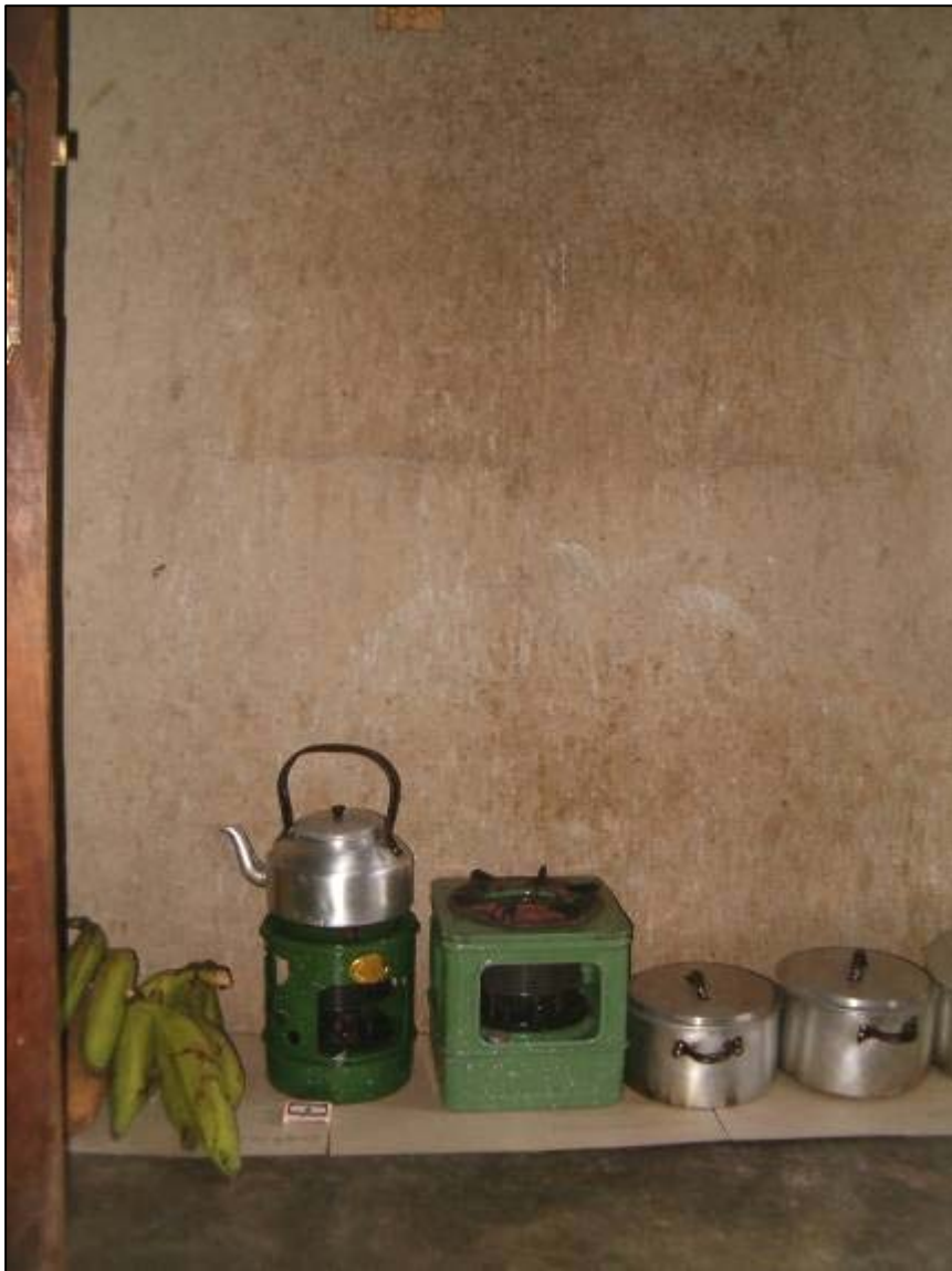
These are the various sizes of kerosene stoves used by the first primary cook in Abraka. The impact of these kerosene stoves could be noticed on the stained wall and the soot on the cooking pots. These are better-quality kerosene stoves.
