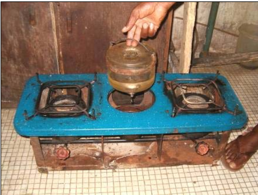
A photo of the double burner kerosene stove having a bottle of kerosene at the centre of the stove; it supplies the cooking fuel to the two burners. This is being used by the second primary cook in Warri to supplement the electric stove and gas cooker (LPG).
