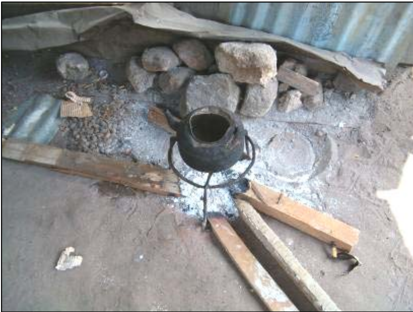
A closer view of the stove being used by the second primary cook in Abraka: a tripod stove with firewood. The kettle has been covered with soot from the firewood fumes.
