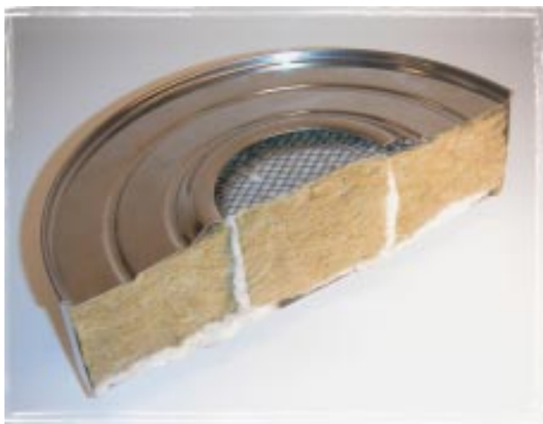
Fig. 3 The fuel canister for the ORIGO® stove is designed for safety and performance. Filled with an absorbent material and holding 1.2 litres of fuel, it is leak-proof, even when held upside down.
