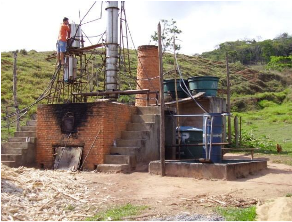
Ponte Nova, Minas Gerais, Brazil. This unit does not have a boiler , it utilizes furnaces.
